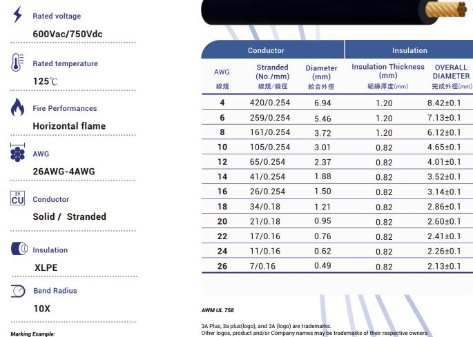
Marking Example: E209277 cUL AWM STYLE 3272 125°C 600V FT2 AWG 3A AWM IA 125°C 600V CAWG FT2 3A LF
