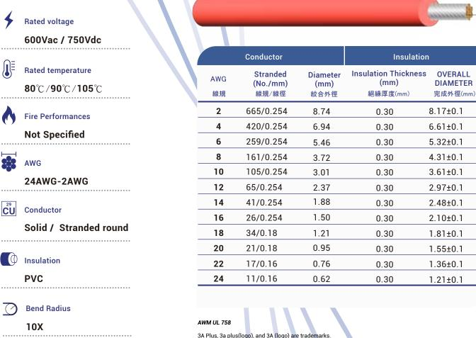
Marking Example: E209277 cUL AWM STYLE 10599 105°C 600V VW-1 . AWG 3A AWM IA 105°C 600V . AWG VW-1 3A LF
